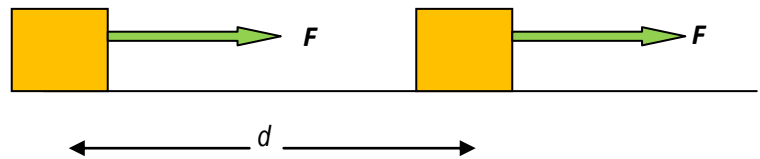
Figure 3.1 Force F is doing work on an object through a distance d .
